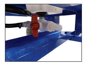
Turn on the Agitation pump to start recirculating water. Water is pulled from the intake drain on the bottom of the tank and returned through three nozzles designed to spray across the bottom of the tank, rotating the liquid vertically in the tank.
