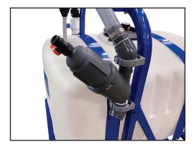
Clean the intake stand-filter by unscrewing the top cap and removing the screen and rinsing to remove any debris.
