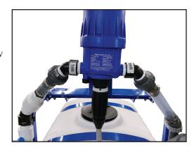
Re-seat the unions into the plumbing with the injector mounted to the mounting bracket and tighten the unions.
